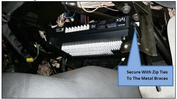
3. **2001 VNM:** The Base Unit is mounted just to the right of the center console, behind the kick panel.
